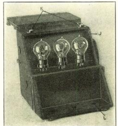
Fig. 2—This Amplifier Is a Complete Unit in Itself and Contains Both A and B Batteries.
